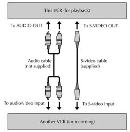
Example 3: When another VCR is S-VHS VCR and when using this VCR as the recording VCR.
